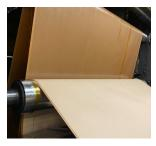
Layers of kraft paper are coated in phenolic resin and a decorative layer is added.
